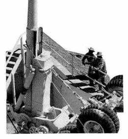
Recent Sandia developments in telemetry instrumentation have made it possible to telemeter information from the test vehicle during its travel through the barrel. These data can be recorded on high-speed tape recorders located in a portable instrumentation trailer adjacent to the gun.
